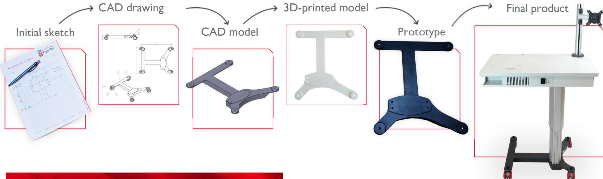
Using modern technologies such as CAD engineering, 3D rendering, 3D printing, and 3D scanning, we create tailored prototypes and accelerate development.
